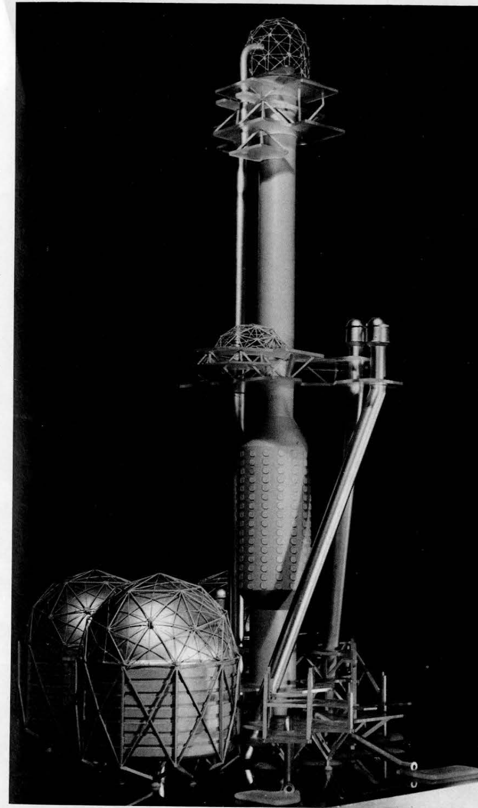
90, 91 Montreal Entertainments Tower project (Peter Cook for Taylor Woodrow, 1963). Elaborately modelled and obsessively drawn out in detail (91), this 600-foot fantasy was firmly grounded in a serious proposal to pre-fabricate the central core for use as a TV transmitter tower all over the world. To make the ludique version proposed for the Montreal Expo of 1967, Peter Cook has hung it with the most admired architectural goodies of the time, from lattice domes to diagonal elevator ducts.
